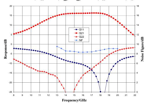
Narrow-band Performance,  $V_{dd}$  = 28 V,  $V_{gg1}$  =  $V_{gg2}$  = -3.4 V,  $I_{dd}$  = 550 mA,  $T_A$  = 25  $^{o}C$
