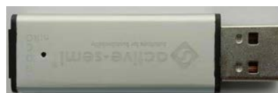
Figure 4 – USB-TO-I2C Dongle Connection
