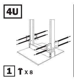
Reverse the mounting ears and secure them as shown using screws provided with your UPS/battery pack.
