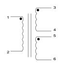
Primary: Secondary: 1 to 2 Series - 3 to 6, Jumper 4 to 5 Parallel - 3 to 6, Jumper 3 to 5 and 4 to 6
