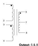
Input (115V): Input 1 & 2 Connect 1&3, 2&4 Input (230V): Input 1 & 4
