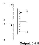
Input (115V): Input 1 & 2 Connect 1&3, 2&4 Input (230V): Input 1 & 4 Connect 2&3
