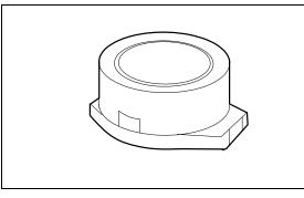
OUTLINE Slim type. Self shielded. Height: 6mm Max. Low resistance. Excellent DC current characteristics.
