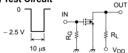
$V_{DD} = -10 \text{ V}$  $R_G = 4.7 \Omega$ Duty  $\leq 1 \%$  $V_{IN}: t_r, t_f < 5 \text{ ns}$
