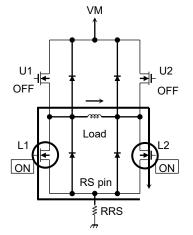
Slow mode A current circulates around the motor coil and this IC.
