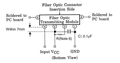
Note 6: Select a resistor value as follows: (with TORX1952A(F))
