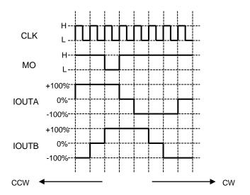
Waveform of MO output: State of pull-up.
