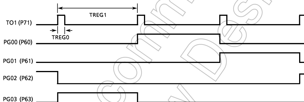
Figure 3.10 (13) Output Waveforms of 4-Phase 1-step Excitation
