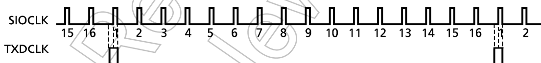
Figure 3.11 (14) Generation of Transmission Clock
