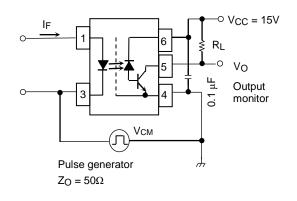
$$\text{CM}_{H} = \frac{1200(\text{V})}{t_{f}(\mu s)}, \text{CM}_{L} = \frac{1200(\text{V})}{t_{f}(\mu s)}$$
