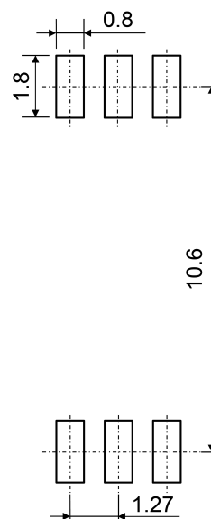
Fig. 16.2 Lead Forming Option (LF4)
