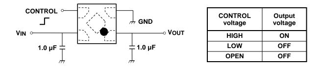
The figure above shows the example of configuration for using a Low-Dropout regulator. Insert a capacitor at VOUT and VIN pins for stable input/output operation. (Ceramic capacitors can be used.)
