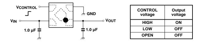
The figure above shows the recommended configuration for using a Low-Dropout regulator. Insert a capacitor at VOUT and VIN pins for stable input/output operation. (Ceramic capacitors can be used.)
