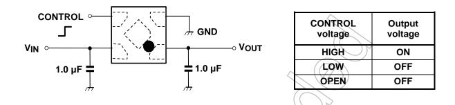
The figure above shows the example of configuration for using a Low-Dropout regulator. Insert a capacitor at VOUT and VIN pins for stable input/output operation. (Ceramic capacitors can be used.)
