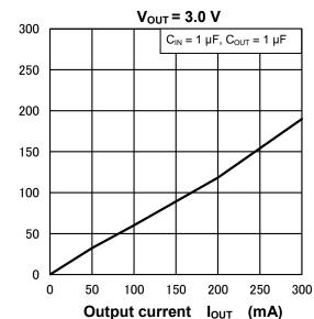
Dropout voltage V<sub>DO</sub> (mV)
