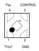
\*Center electrode should be connected to GND or Open
