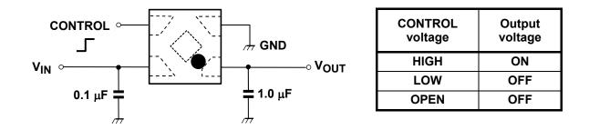
The figure above shows the recommended configuration for using a Low-Dropout regulator. Insert a capacitor at  $V_{OUT}$  and  $V_{IN}$  pins for stable input/output operation. (Ceramic capacitors can be used).
