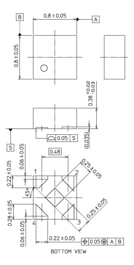
0.04 mm (typ.) unevenness exists along the edges of the back electrode to increase shear after soldering.
