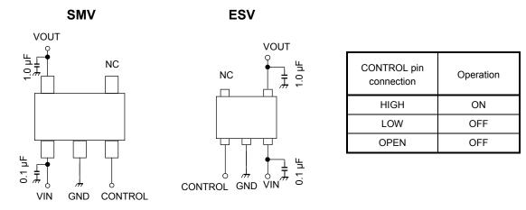
The figures above show the examples of configuration for using a Low dropout regulator. Insert a capacitor at V<sub>OUT</sub> and V<sub>IN</sub> pins for stable input/output operation. (Ceramic capacitors can be used).
