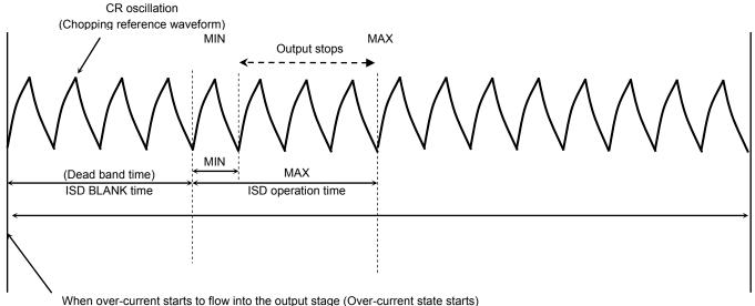
which over-current starts to now into the output stage (Over-current state starts)
