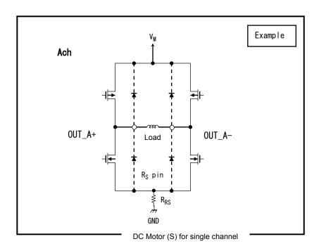
O ... Indicates an IC output pin connected to a motor.
