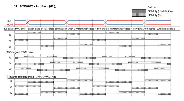
In this timing chart, the reverse rotation brake is indicated without current limit.
