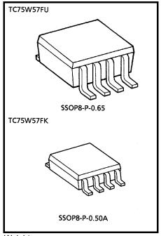
Weight SSOP8-P-0.65: 0.021g (typ.) SSOP8-P-0.50A: 0.01g (typ.)
