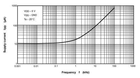
The above characteristics curves are presented for reference only and not guaranteed by production test, unless otherwise noted.
