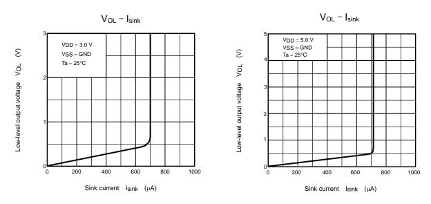
The above characteristics curves are presented for reference only and not guaranteed by production test, unless otherwise noted.
