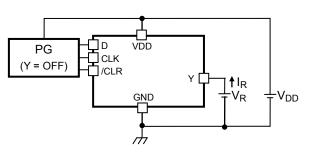
7.  $t_{pHL}$  (CLK),  $t_{pLH}$  (CLK),  $t_{pHL}$  (/CLR)
