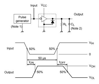
Note 1: Pulse width 50 µs, Duty cycle 10% Output impedance 50  $\Omega$ , t<sub>r</sub> ≤ 5 ns, t<sub>f</sub> ≤ 10 ns, V<sub>IH</sub> = 5.0 V
