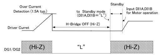
CAUTION: Over Current Detection circuits is only intended to provide temporary protection against irregular conditions such as an output short-circuit; they do not necessarily guarantee the complete IC safety.
