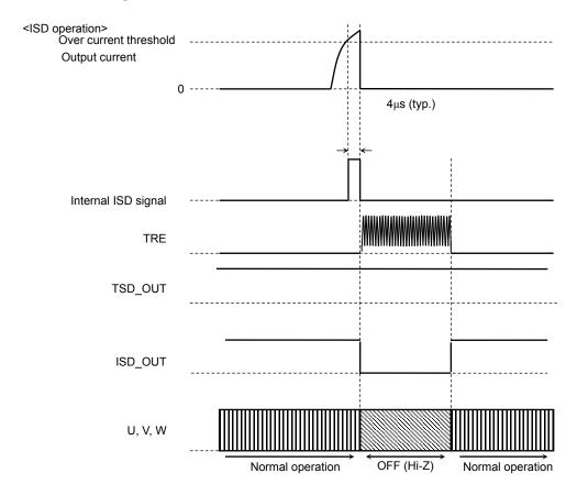
Note: The ISD circuit is activated if the absolute maximum current rating is violated. Note that the circuit is provided as an auxiliary only and does not necessarily provide the IC with a perfect protection from damages due to overcurrent caused by power fault, ground fault, load-short and the like.
