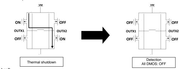
•When over temperature is detected:
