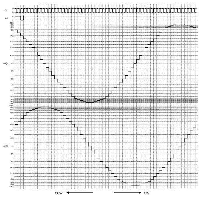
Waveform of MO output: State of pull-up.
