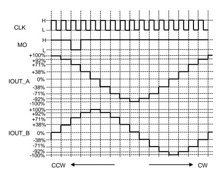
Waveform of MO output: State of pull-up.
