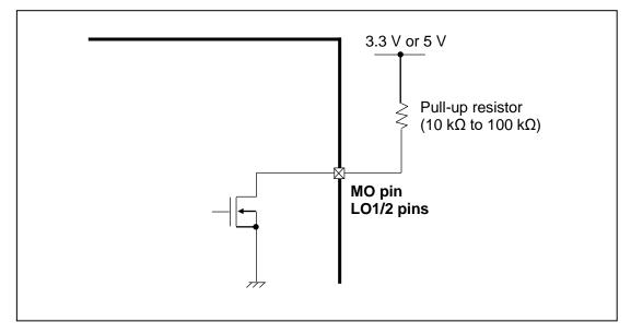
The equivalent circuit diagrams may be simplified or omitted for explanatory purposes.
