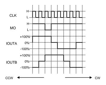
Waveform of MO output: State of pull-up.
