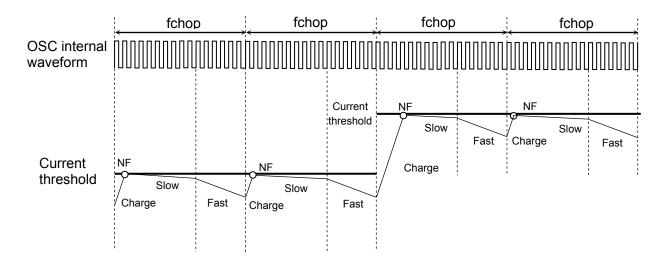
· When the next step's current threshold is less than that of the previous step
