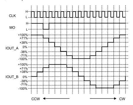
Waveform of MO output: State of pull-up.
