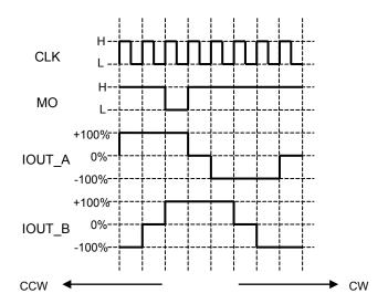
Waveform of MO output: State of pull-up.
