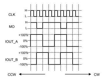
Waveform of MO output: State of pull-up.
