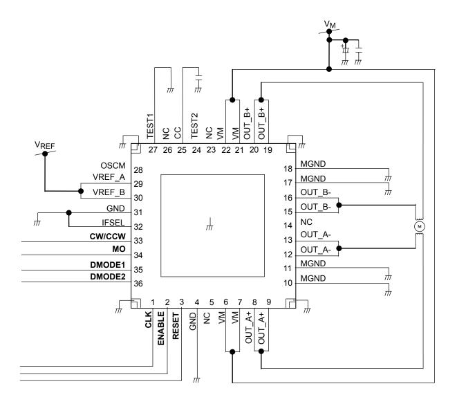
Heat dissipation PAD (4 corners and the center part) on the back of the package is recommended to connect to the GND of the board for improved heat dissipation.
