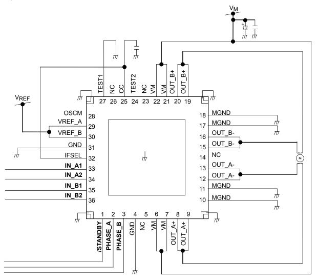
Heat dissipation PAD (4 corners and the center part) on the back of the package is recommended to connect to the GND of the board for improved heat dissipation.
