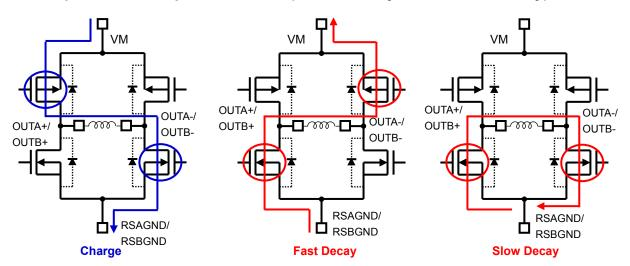
Note: Fixed value of 400 ns (design value) is prepared at the switching timing of MOSFET output to avoid any flow-through current. The equivalent circuit diagrams may be simplified or omitted for explanatory purposes.
