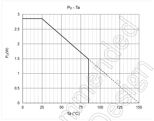
When mounted on the board (JEDEC 4 layers)
