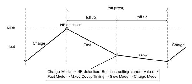
If the output current is zero-detected during Fast mode, the output becomes High impedance.
