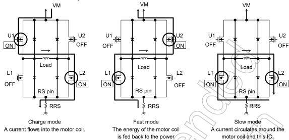
**Operation Function of Output Transistor**
