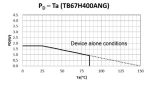
This value is dependent on a substrate pattern and mounting conditions. Moreover, when ambient temperature is high, permissible power consumption becomes small.
