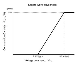
Note: The conduction time is reduced by the dead period. (carrier cycle×92% – Td×2)
