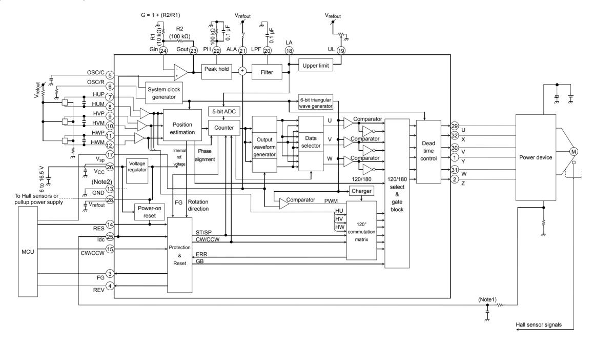
Note1: Connect to ground as necessary to prevent IC malfunction due to noise.
