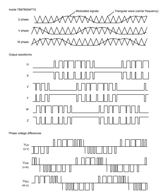
In sine-wave drive mode, the amplitude of the modulated signals varies with the Vsp voltage and the motor speed changes with the conduction duty cycle of the output waveforms. (See the Sine-wave drive mode diagram on page 14.)
