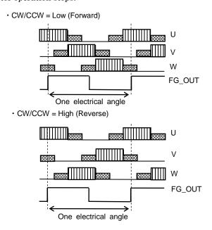
2) Output of rotation speed signal: FG\_OUT pin
