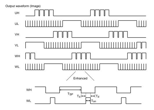
TSP: Changeable by VSP. (The condition in this figure: VSP = 5.4 V (typ.)), Ton = 18/fosc, Td = 9/fosc.
