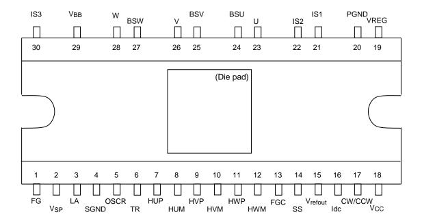
Note: Die pad on the package surface and PGND are connected. When using the heat sink, handle it not to short to the IC pins. When applying the different potential with GND level to the heat sink, insulate with die pad and the heat sink.
