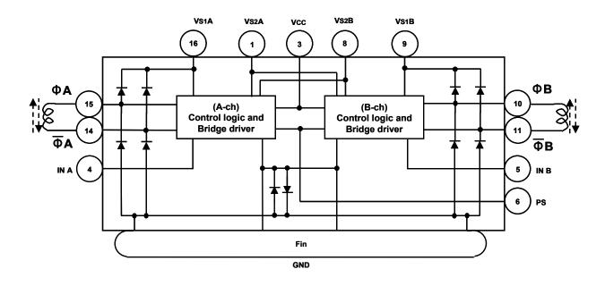
Note: TB6674FG: Terminals 2, 7, 12, and 13 are NC. TB6674FG: The heat fin is connected to GND.
