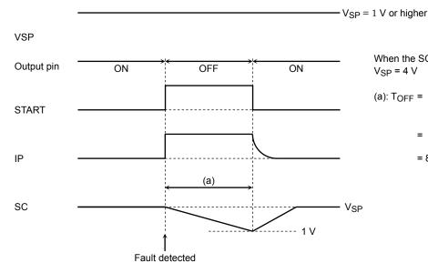
When the SC pin capacitor = 0.47  $\mu F$  and  $V_{SP}$  = 4 V
