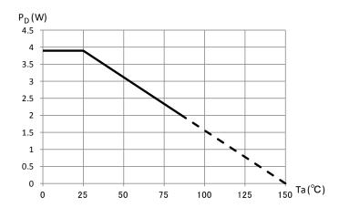
Measured on a board (100 mm  $\times$  100 mm  $\times$  t1.5 mm, Double-layers) Rth (j-a) = 32°C/W
