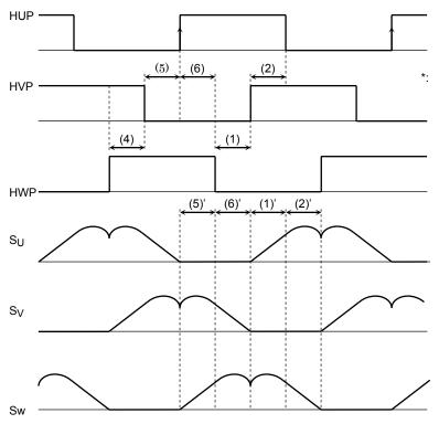
Though the HUP, HVP and HWP pins are Hall effect inputs, they are indicated as square waveforms for the sake of simplicity.
