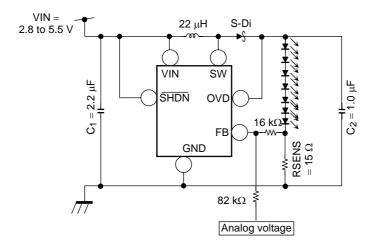
(3) Input PWM signal with filtering to FB terminal
