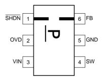
Note: This IC could be destroyed in some case if amounted in 180° inverse direction. Please be careful about IC direction in mounting.
