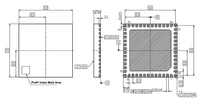
Backside heatsink: 5.4 mm  $\times$  5.4 mm Corner chamfers: C0.5 Chamfer radius: 3-R0.2
