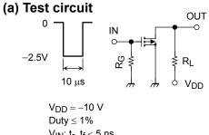
$V_{IN}\text{: }t_{r}\text{, }t_{f}<5\text{ ns}$  $(Z_{out} = 50 \Omega)$ Common Source  $Ta = 25^{\circ}C$
