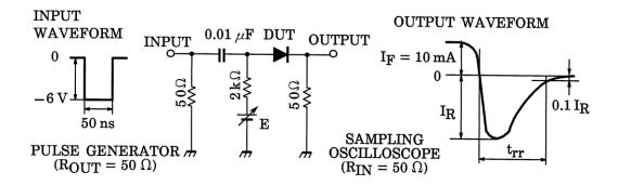
Fig.1 Reverse Recovery Time (t<sub>rr</sub>) Test Circuit
