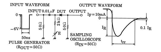
Fig.1 Reverse Recovery Time (trr) Test Circuit
