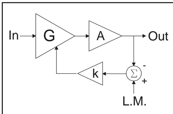
Figure 2. Feedback compressor.
