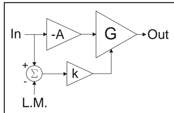
Figure 3. Feedforward expander.
