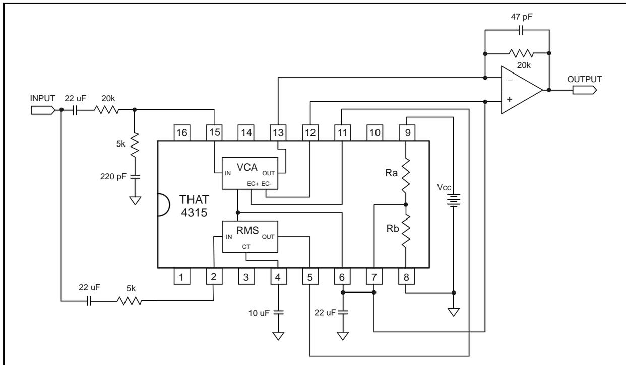
Figure 5. 4315 Typical Application Circuit - 1:2 Expander
