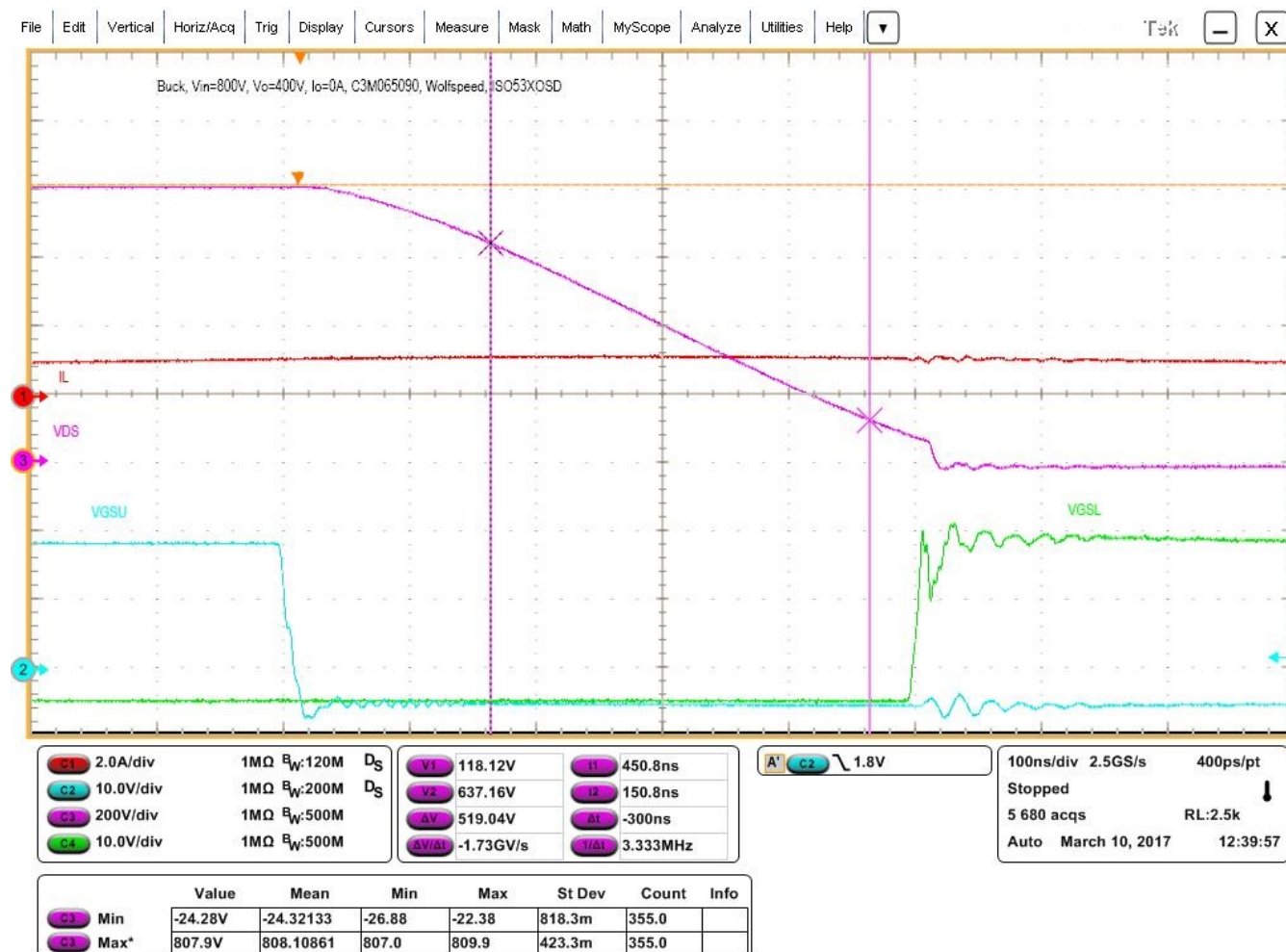
Figure 11. Expanded Soft Switching Waveforms During Vds Fall
